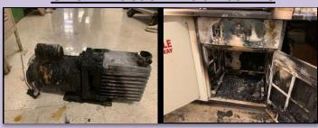
The fire occurred when a power switch ignited vapors that had accumulated in a vacuum pump cabinet.
