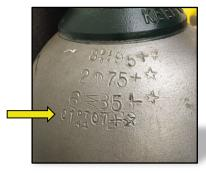
This tank was last inspected on 01/2007, without a star the tank is good for 5 years, with the star this tank is good for 10 years. The date should tell you to stop using this tank and return it to the company by January 2017. Take time today to look at tanks in your lab, how many should be returned soon, how many should be returned today?!
