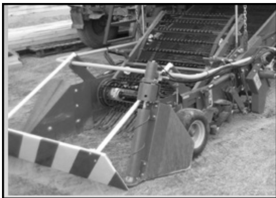
Combing-oscillating-lifting cutter bar type header
