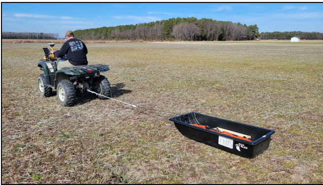
Figure 3: An EM38 being pulled in a plastic sled to minimize contact with metal. A GPS unit is mounted to the 4-wheeler to georeference the EC a measurements (photo: Jarrod Miller).
