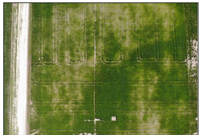
Figure 5: A visual camera can reveal differences in plant growth not easily spotted from the ground..
