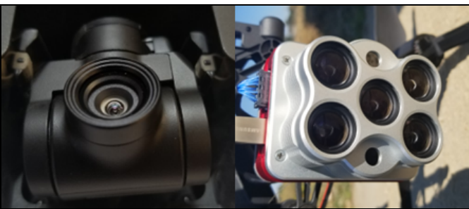
Figure 3: A visual camera (left) captures the spectrum the human eye while a multispectral (right) will have several lenses capturing specific wavelengths of light (photo: Jarrod Miller).
