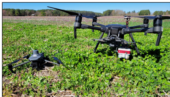
Figure 1: Two rotary drones with four propellers, making them quadcopters, the most common drone on the market (photo: Jarrod Miller).
