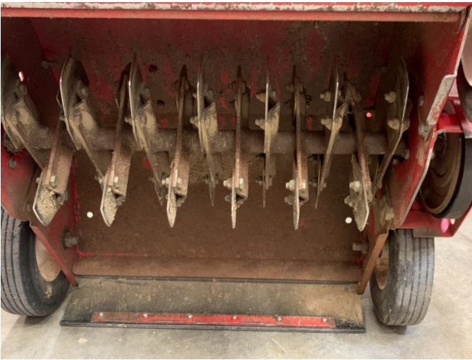
Fig. 2. Evenly spaced, spinning vertical blades of a verticutting machine
