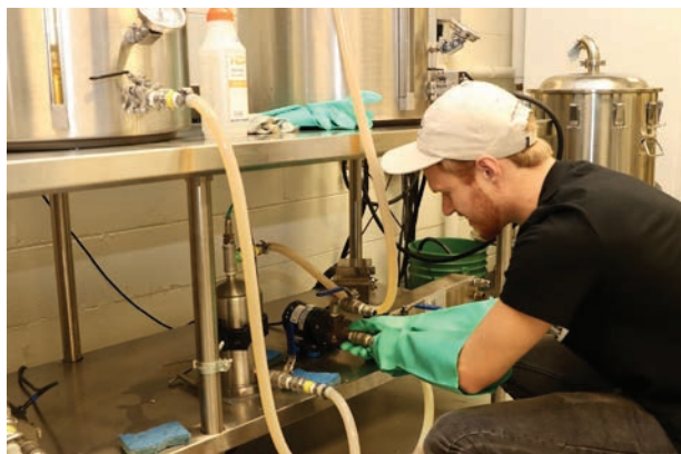
Food Science senior Sam Hete is shown connecting the tubing to an electrical pump to start the lautering process for a recent batch of pale ale.
