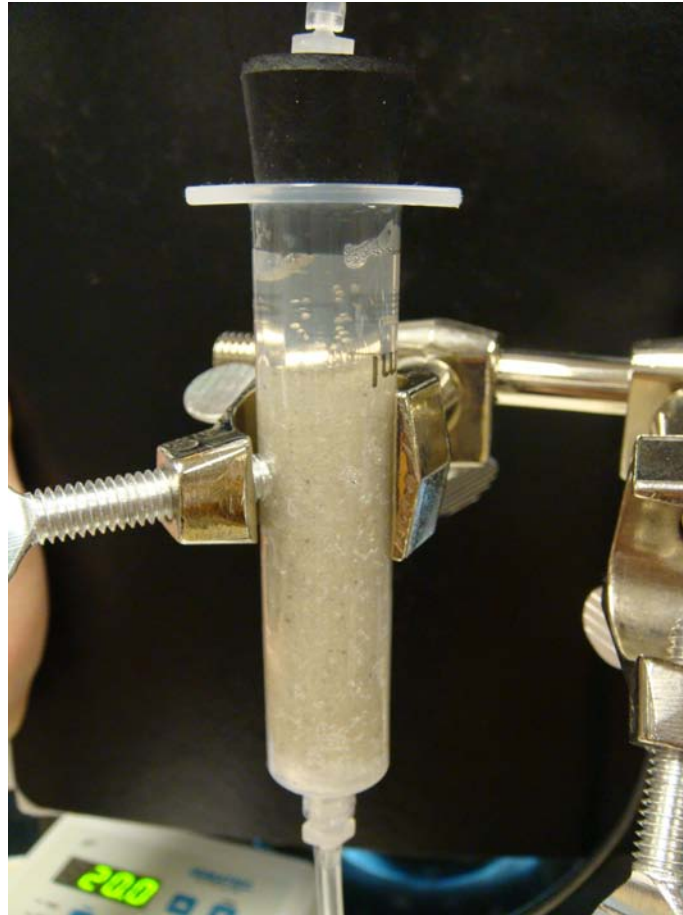
Figure 3.1 A column packed with quartz sand. The influent solution was injected by a peristaltic pump at the bottom of the column and collected from the top. The effluent was sampled daily throughout the experiments.
