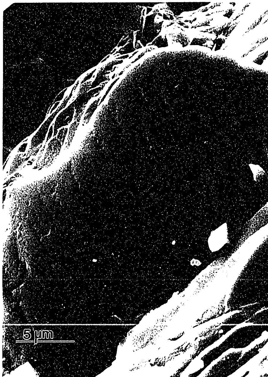
Figure 3.5 SEM image of a clinopyroxene surface weathered at pH 5. Side-by-side alignment of etch pits are visible along the basal lamellae.
