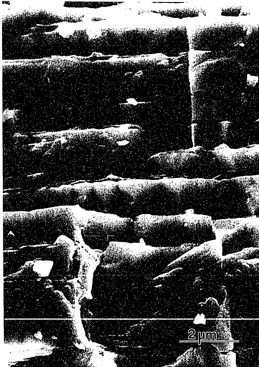
Figure 3.11 SEM image of a clinopyroxene surface weathered at 20 mM citric acid. Etching of the surface is clearly visible along basal lamellae.
