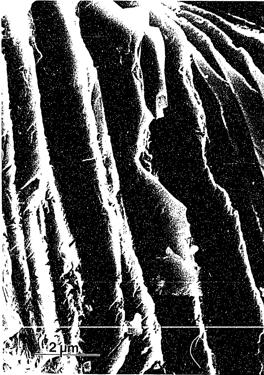
Figure 3.13 SEM image of a clinopyroxene surface weathered at 20 mM citric acid. Note the formation of etch pits along the basal lamellae.
