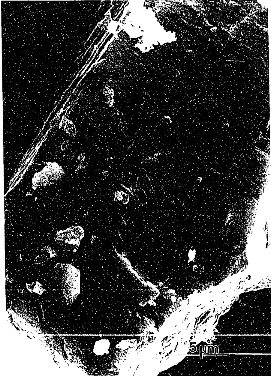
Figure 3.12 SEM image of a clinopyroxene surface weathered at 20 mM oxalic acid. Etch pits are visible along the basal lamellae although not as extensive as Fig. 3.11.
