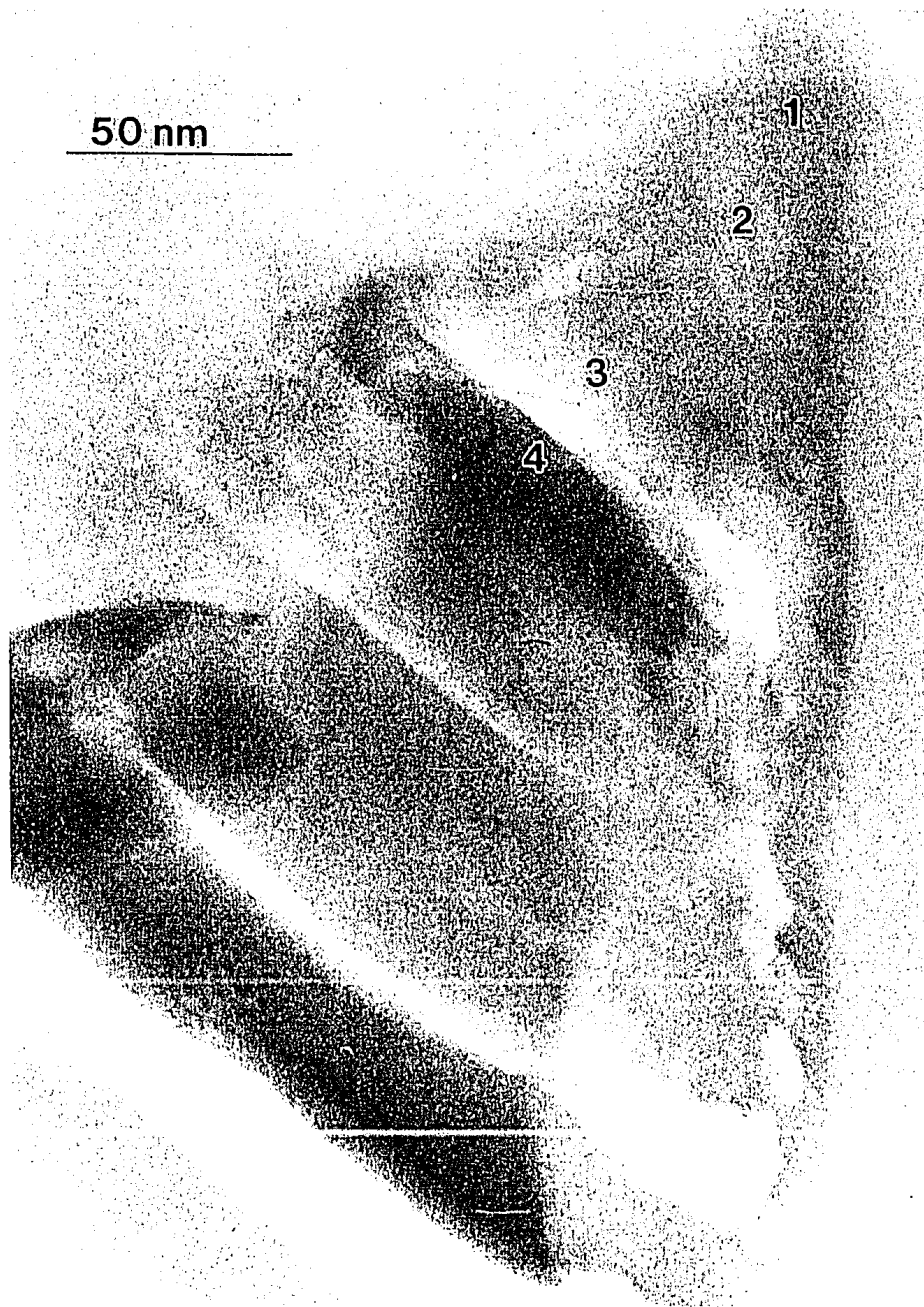
Figure 2.14 High magnification TEM image of Fig. 2.13 showing the four regions where the EDS spectra were obtained.
