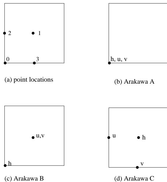
Figure 4: Staggered grid definition.
