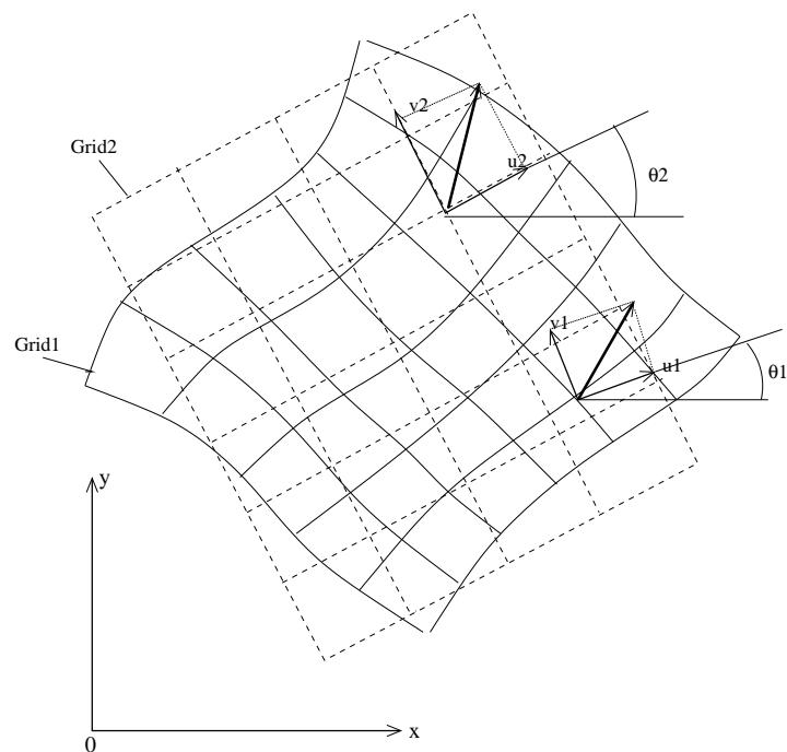
Figure 3: Example of module grids in geographical reference coordinates.
