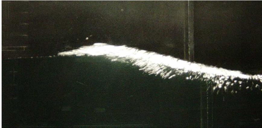
**Figure 1.1:** Laboratory generated spilling breaker. Photograph provided by Dr. B. K. Haus and Dr. M. A. Donelan, Rosenstiel School of Marine and Atmospheric Science, University of Miami.
