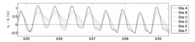
Figure 1. Measured water levels during (3/25-3/27) and shortly after (3/27-3/29) the surge event, less their respective means, with distance landward increasing from Site A to Site F
