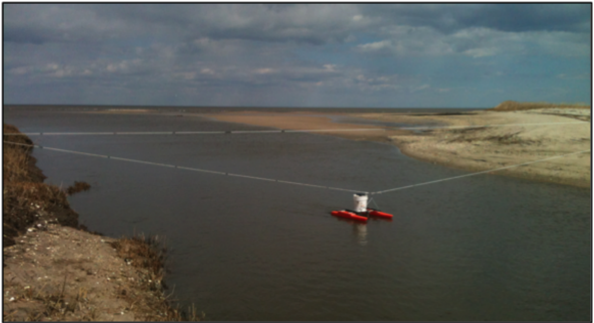
Figure 2.14: Deployment of a catamaran vessel at mouth, near Site A, used to measure cross-sectional bathymetry. The picture is oriented in the direction looking towards Delaware Bay. The locations of the measured points are given in Figure 2.9.
