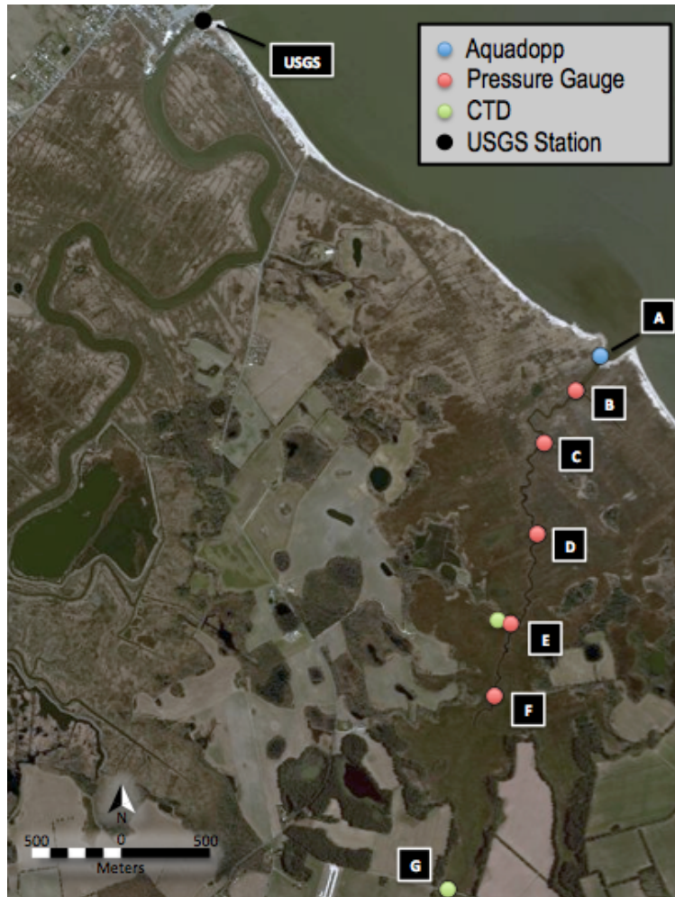
Figure 2.6: Layout of instrument locations in Brockonbridge Marsh. The black dot near the upper left corner marks the location of a USGS tidal and discharge gauge station, at the mouth of the Murderkill River. The location labeled Site G is the aforementioned small bridge in the discussion of site selection. ( Satellite imagery is from ESRI. )
