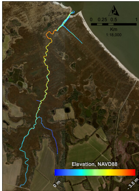
Figure 2.8: Interpolated bathymetry of Brockonbridge Gut and its navigable branches, computed with the kriging technique. (a) The entire Brockonbridge Marsh up to the bridge; (b) Enlargement of domain near the mouth. The grid spacing is 1 meter. The maximum search radius was 3 meters, with a maximum of 10 nearest points used during interpolation. Note: the satellite image was taken prior to the dates during which the bathymetric surveys were conducted, at which time the sand bank near the mouth was further north; however, the satellite imagery serves as a good frame of reference, and is thus included. (Satellite imagery is from ESRI.)
