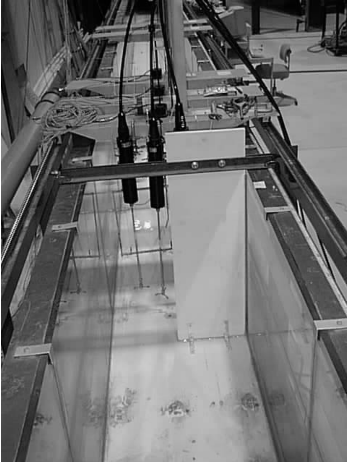
Figure 2.2: Digital photograph showing the breakwater and instrument setup.
