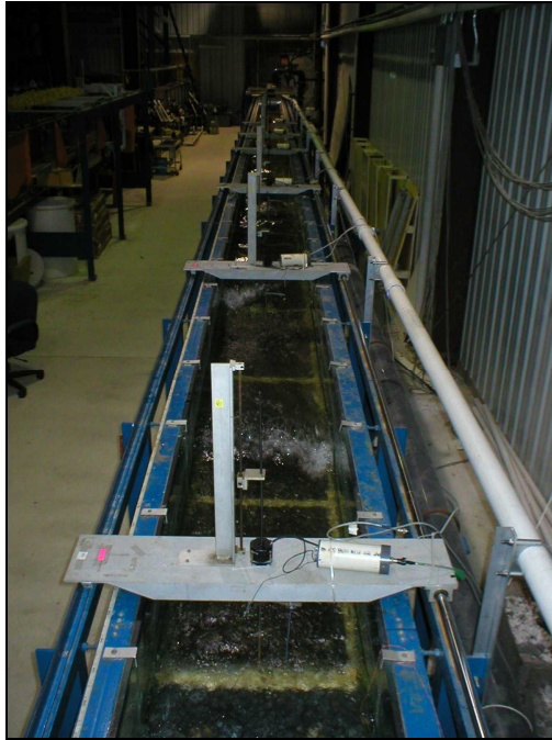
Figure B1 Picture of Gage Setup Facing Wave Maker from Above Ramp
