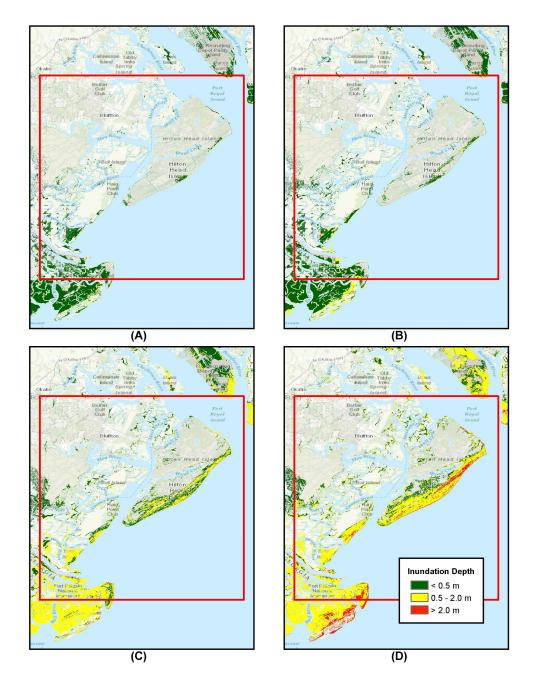
Figure 10: Inundation depth for SA\_1arc\_4 domain, A) SMF, B) Coseismic Envelope, C) CVV 80 km<sup>3</sup> slide, and D) CVV 450 km<sup>3</sup> slide. Red box depicts SA\_1arc\_4 domain boundaries.
