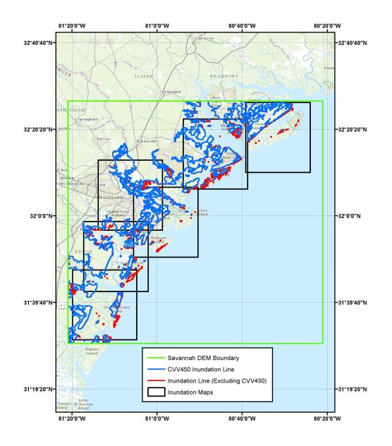
Figure 16: Tsunami inundation line for Savannah NGDC DEM area based on tsunami sources simulated in this project. The red line shows the inundation line for the envelope of all sources excluding CVV450. The blue line demontrates the CVV450 inundation line. The black boxes show the location of the inundation maps discussed in Section 5.
