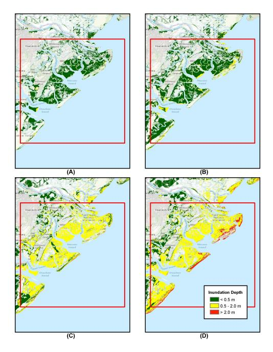
Figure 9: Inundation depth for SA\_1arc\_3 domain, A) SMF, B) Coseismic Envelope, C) CVV 80 km<sup>3</sup> slide, and D) CVV 450 km<sup>3</sup> slide. Red box depicts SA\_1arc\_3 domain boundaries.
