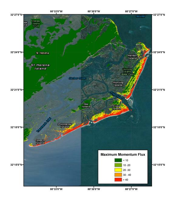
Figure 13: (Maximum Momentum Flux Map for Fripp Island during CVV450 tsunami (Colorbar values are in  $m^3/s^2$ )
