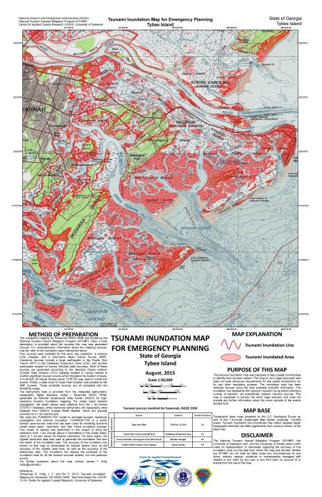
Figure 19: Inundation map for emergency planning for Tybee Island, GA in 1:50,000 scale. The inundated area is shown in red, and the thick red line represents the inundation line for this particular area.
