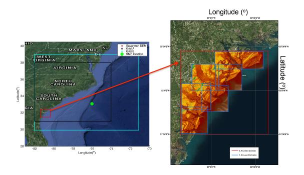
Figure 4: The sequence of grid nesting. The figure on the left depicts the Grid A and B as well as the location of the Savannah DEM. The figure on the right show the 1 arc-sec grids described in Table 1.
