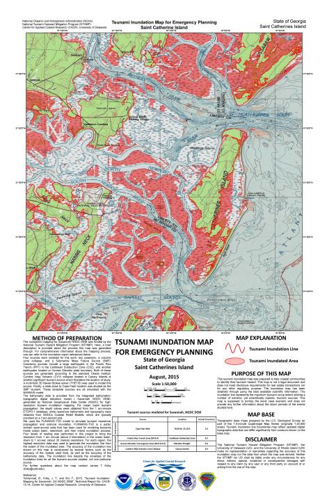
Figure 22: Inundation map for emergency planning for Saint Catherines Island, GA at 1:50,000 scale. The inundated area is covered in red, and the thick red line represents the inundation line for this particular area.
