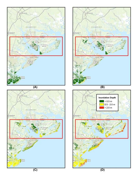
Figure 12: Inundation depth for SA\_1arc\_6 domain, A) SMF, B) Coseismic Envelope, C) CVV 80 km<sup>3</sup> slide, and D) CVV 450 km<sup>3</sup> slide. Red box depicts SA\_1arc\_6 domain boundaries.
