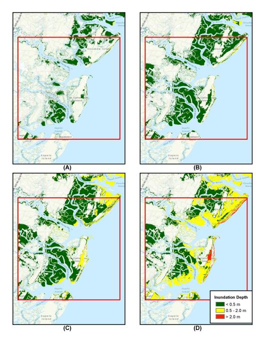
Figure 7: Inundation depth for SA\_1arc\_1 domain, A) SMF, B) Coseismic Envelope, C) CVV 80 km<sup>3</sup> slide, and D) CVV 450 km<sup>3</sup> slide. Red box depicts SA\_1arc\_1 domain boundaries.
