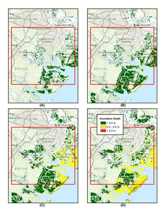
Figure 8: Inundation depth for SA\_1arc\_2 domain, A) SMF , B) Coseismic Envelope, C) CVV 80 km<sup>3</sup> slide, and D) CVV 450 km<sup>3</sup> slide. Red box depicts SA\_1arc\_2 domain boundaries.
