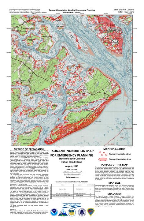
Figure 18: Inundation map for emergency planning for Hilton Head Island, SC in 1:50,000 scale. The inundated area is shown in red, and the thick red line represents the inundation line for this particular area.
