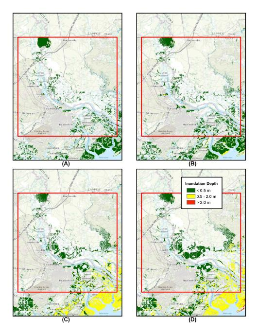
Figure 11: Inundation depth for SA\_1arc\_5 domain, A) SMF, B) Coseismic Envelope, C) CVV 80 km<sup>3</sup> slide, and D) CVV 450 km<sup>3</sup> slide. Red box depicts SA\_1arc\_5 domain boundaries.
