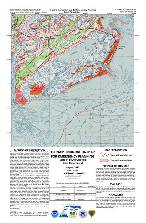
Figure 17: Inundation map for emergency planning for Saint Elena, SC in 1:50,000 scale. The inundated area is covered in red, and the thick red line represents the inundation line for this particular area.
