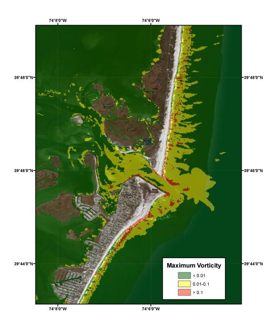
Figure 14: Maximum Vorticity map for the area around Barnegat inlet
