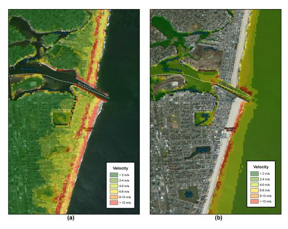
Figure 13: (a) Maximum Velocity map for inundated area around Manasquan inlet (SMF1) (b) Maximum Velocity map for Manasquan Inlet for offshore areas (SMF1)
