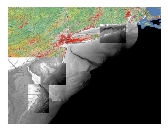
Figure 2: Mosaic of DEM and land use information based on NGDC tsunami DEM's, FEMA DEM's for Region 2 and Region 3 hurricane studies, and National Land Cover Data. Work covered by this project will provide maps for the Ocean City, Atlantic City and Montauk DEM's (smallest highlighted areas) and Myrtle Beach, SC using NGDC DEM's, and the remainder of the western half of Long Island using FEMA DEM's.
