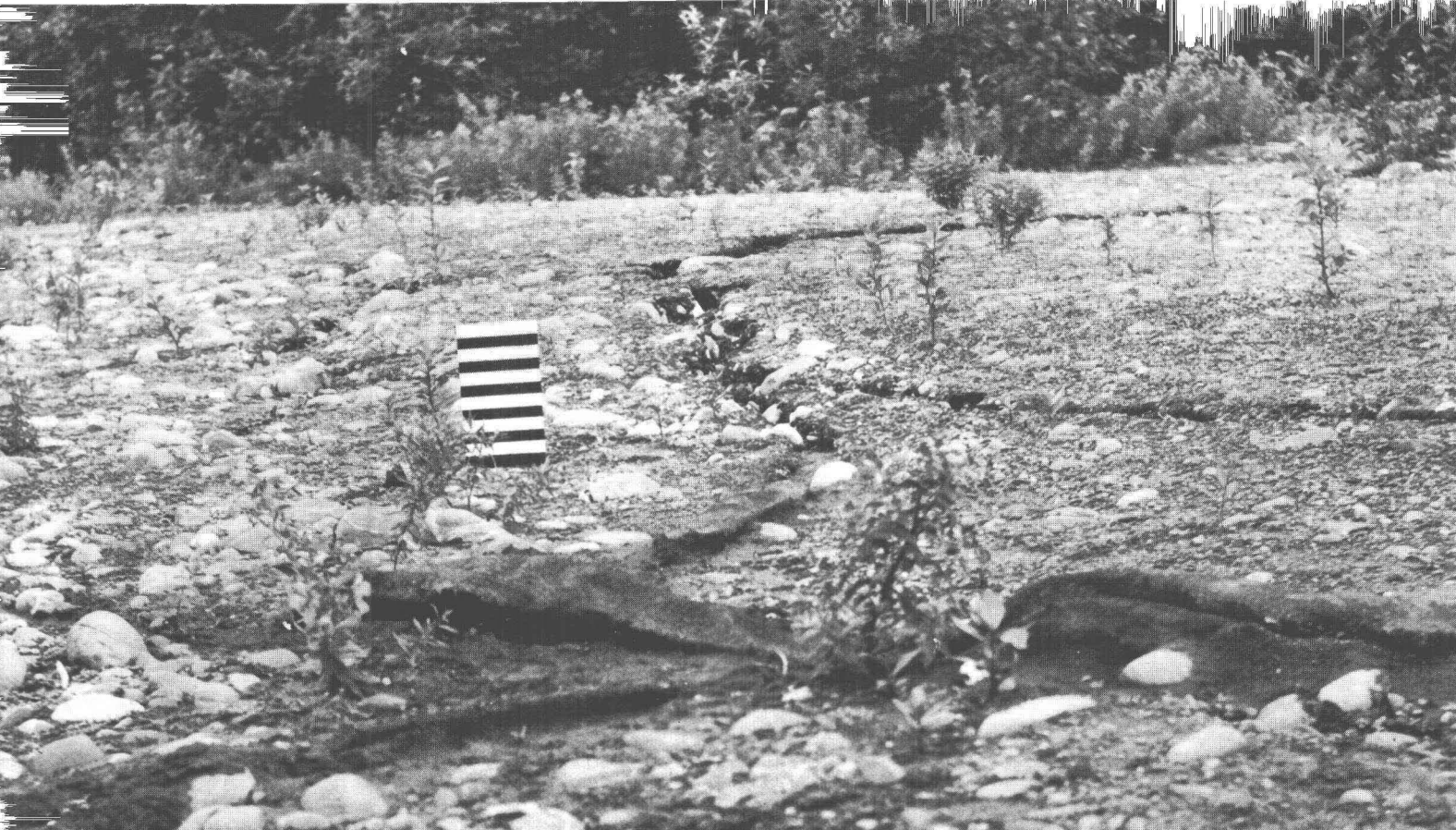
14.—Zone of intersection between longitudinal fissures (foreground) and transverse fissure (background). Note increasing evidence of sand ejection along transverse fissure as it approaches longitudinal-fissure complex. Scale is 1 foot.
