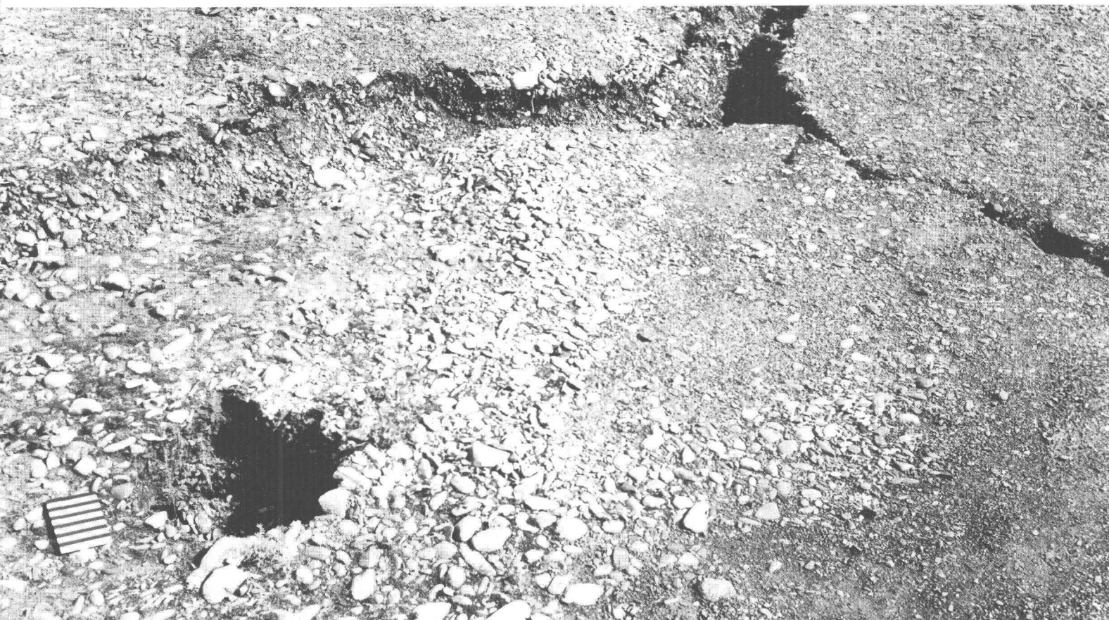
15.—Collapse pit in a graben on the flank of a set of longitudinal fissures. Scale is 1 foot.
