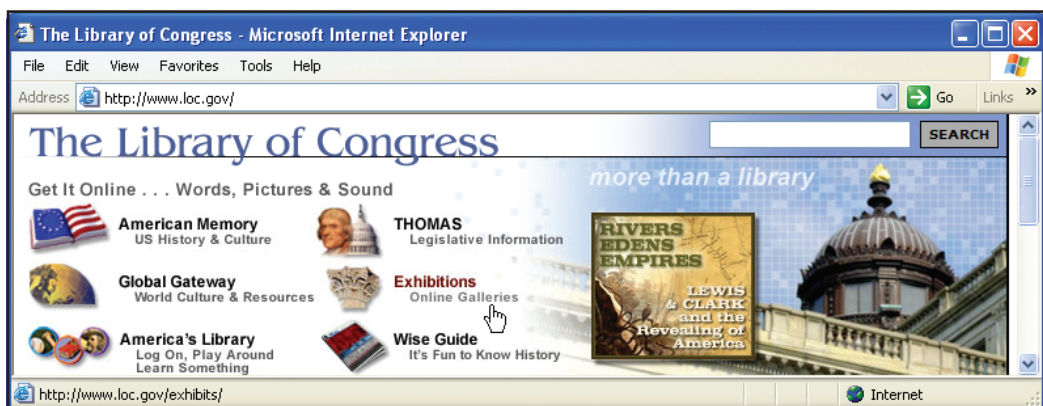
FIGURE 2-13 A rollover effect created with JavaScript at the Library of Congress. To try this effect, go to www.loc.gov and move your cursor over the menu choices. Notice that the photo on the right changes as you mouse over the choices. ■
