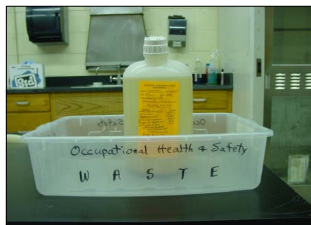
LDPE Nalgene Carboy in a secondary containment bin
