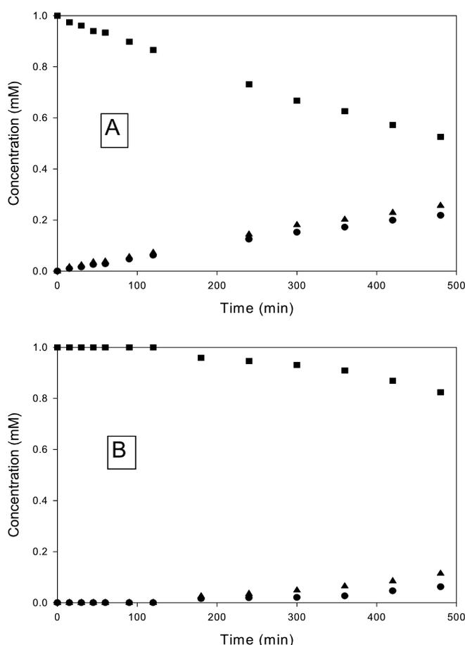
**Figure 2.** Reactivity of (A) VCPO and (B) VBPO toward TNT (■) in aqueous systems (pH 8.0), producing trinitrobenzyl alcohol (●) and trinitrobenzene (▲). Reaction conditions are described in the text.
