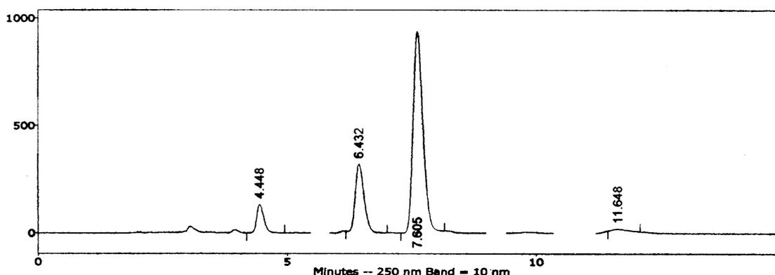
**Figure 1.** HPLC trace for the vanadium chloroperoxidase (60 μM) reaction with TNT (10 μM) containing 10 mM KBr, 2 mM H<sub>2</sub>O<sub>2</sub>, and 1 mM Na<sub>3</sub>VO<sub>4</sub>. Chromatogram represents product distribution after 24 h. Vanadium bromoperoxidase catalysis gave a similar reaction profile, albeit at lower yields.
