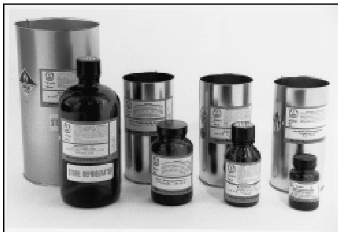
Fig. 1 Pyrophoric reagents may be packed in a variety of containers.
