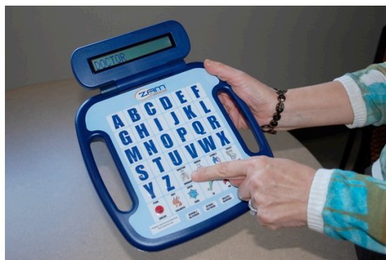
Caption: Demonstrating the front of the Zam Communicator with LCD screen displaying the text "doctor"
