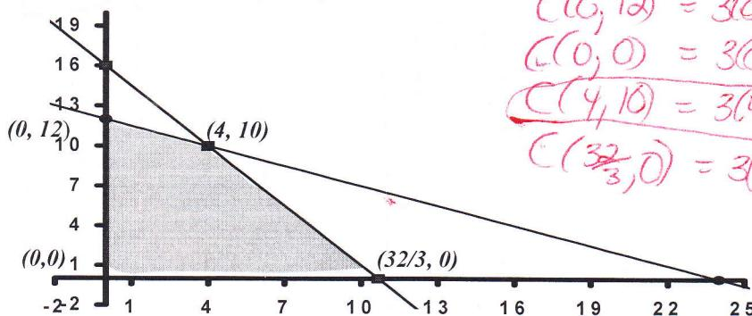
$$\begin{aligned}C(6, 12) &= 3(6) + 5(12) = 60 \\C(0, 0) &= 3(0) + 5(0) = 0 \\C(4, 10) &= 3(4) + 5(10) = 62 \\C\left(\frac{32}{3}, 0\right) &= 3\left(\frac{32}{3}\right) + 5(0) = \frac{96}{3} = 32\end{aligned}$$
