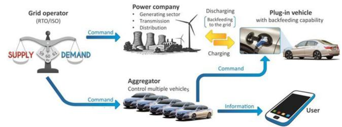
Figure 2. Overall configuration of V2G system
