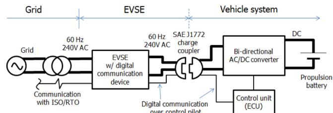
Figure 4. Configuration of the V2G-capable vehicle
