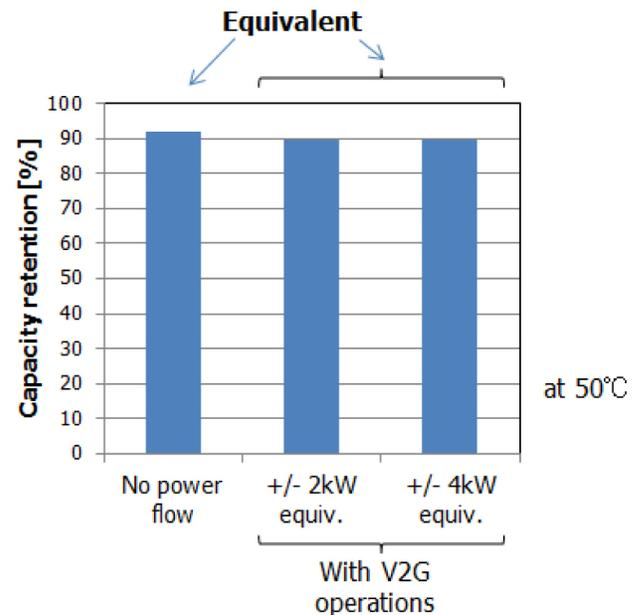
Figure 7. Capacity retention rate after high temperature durability tests, showing near equivalence in capacity whether or not V2G is added.
