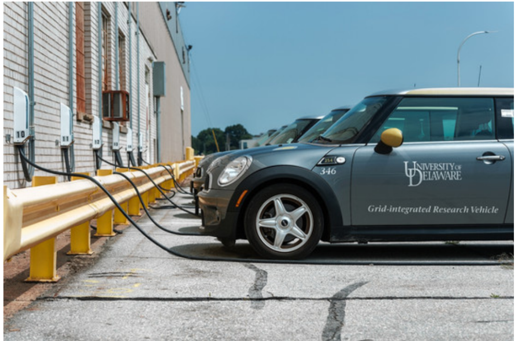
University of Delaware electric cars act as a reserve for the power grid, discharging electricity when needed.
