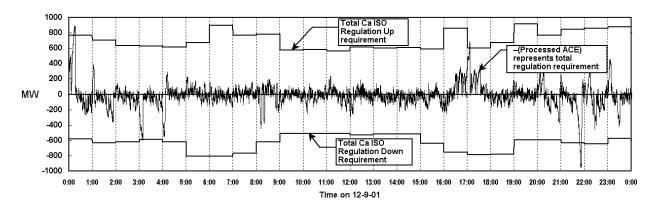
Figure 10. Total regulation capacity (procured+self) and regulation dispatch requirement (represented by -PACE).
