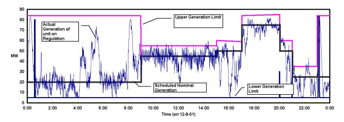
Figure 8. Full day power profile of a hydro power plant on regulation. Also shown are the scheduled nominal generation and upper and lower limits.
