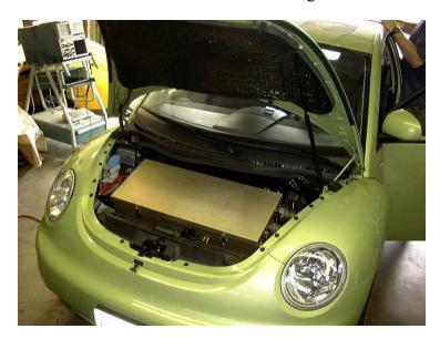
Figure 7. AC150 Gen-2 drivetrain with bi-directional grid power capability installed in Beetle EV
