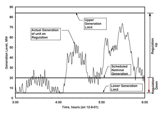
Figure 4. Example power generation profile of a hydro plant providing grid regulation (data source: Cal ISO).
