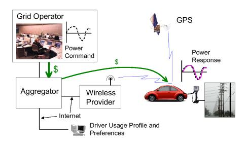
Figure 6. Architecture of vehicle-based grid regulation system.
