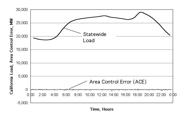
Figure 3. Example showing relative magnitude of system total load and Area Control Error (ACE) for March 14, 2001.
