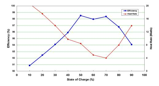
Figure 26. Battery cycle efficiency data as a function of SOC (source: NREL)
