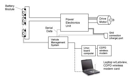
Figure 19. Architecture of vehicle power system with V2G capability.
