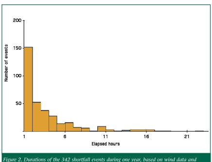
Figure 2. Durations of the 342 shortfall events during one year, based on wind data and assuming that power is combined from eight dispersed wind sites
