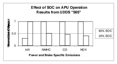
Figure 11. Effect of Battery SOC
