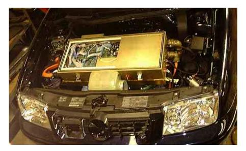
Figure 3. Electric Drive System Installed
