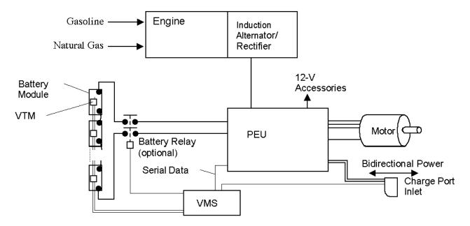
Figure 1. Power System Architecture
