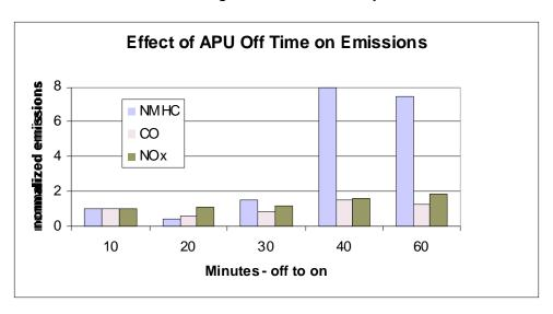
Figure 10. Effect of APU Off Time
