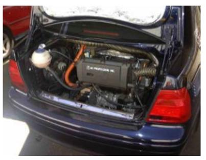
Figure 7. APU Installed
