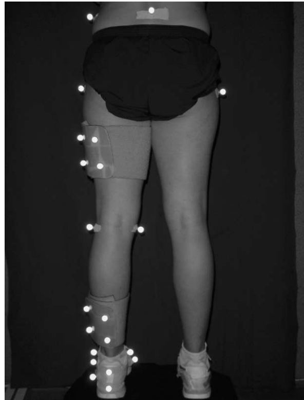
Fig. 1. Retroreflective marker placement on the tested lower extremity.
