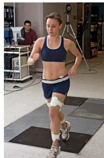
Allison Altman, a PhD student in the Biomechanics and Movement Science Program and member of Davis's lab, runs across force plates in the motion analysis lab (MAL).
