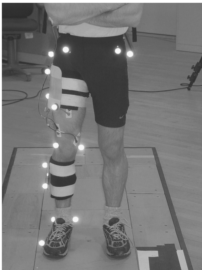
Figure 1. Retroreflective marker placement. The medial knee and ankle markers and the left and right ASIS markers were only used during a static trial (to configure each subject with the global coordinate system) and were removed before the subject performed the dynamic landing trials. ASIS, anterior-superior iliac spine.
