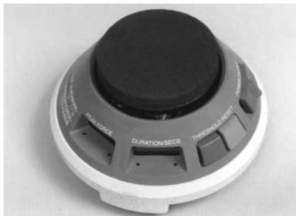
Figure 1 Handheld dynamometer used to test muscle strength of the shoulder.
