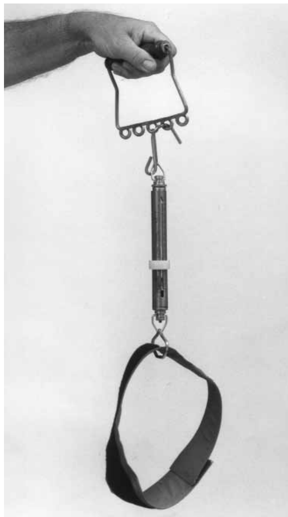
Figure 2 Spring-scale dynamometer used to test muscle strength of the shoulder.
