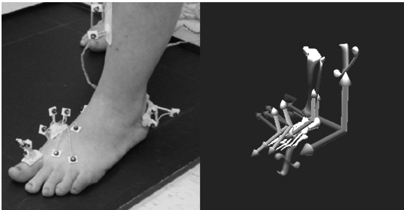
FIGURE 1. Infrared emitting diode (IRED) sets and subsequent coordinate systems used to establish a 5-segment foot model.
