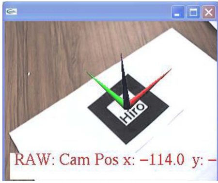
Fig. 5 A single camera detects six degree-of-freedom information of a marker
