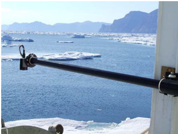
Figure 9. Cameras used to photograph the ice in the ship's path. That at the left is down-looking and provides images for measurement of ice thickness. That at the right photographs floes ahead of the ship before their impact.
